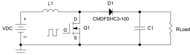
**Figure 1. Boost Converter:** One of the most traditional uses of the Schottky rectifier is in the boost converter, which requires a low-loss rectification element. The CMDFSH Series has been designed to highlight the main qualities of Schottky rectifiers in a space-efficient package; including a low forward voltage drop, fast turn-on time, and extremely fast recovery time. These attributes make the CMDFSH Series an excellent boost rectifier choice for any boost converter system.
