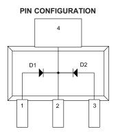
LEAD CODE: 1) Anode D1 2) Cathode D1, D2 3) Anode D2 4) Cathode D1, D2
